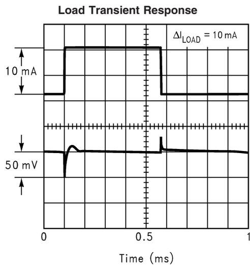
**LM4140 Typical Performance Characteristics** Unless otherwise specified,  $T_A = 25^\circ\text{C}$ , No Load,  $C_{OUT} = 1\mu\text{F}$ ,  $V_{IN} = 3.0\text{V}$  for LM4140-1.024 and LM4140-1.250, and 5V for all other voltage options.  $V_{IN} = V_{EN}$ . (Continued)
