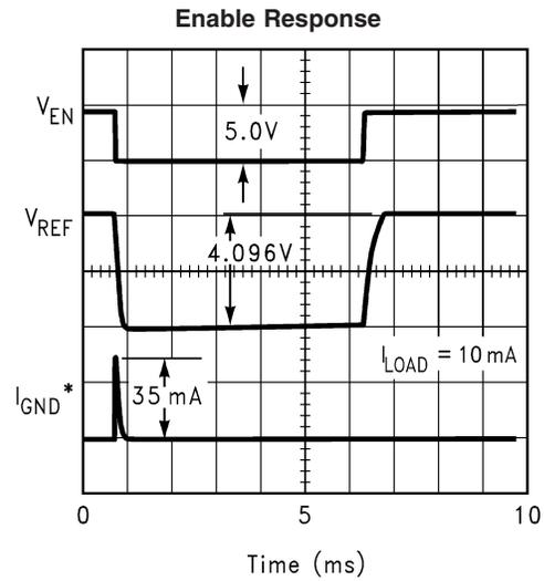
\* The  $1\mu\text{F}$  output capacitor is actively discharged to ground. See ON/OFF Operation section for more details.
